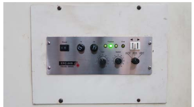
Controller 86B is installed on Screen Printing Machine by Insertion
